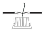
3. PUSH THE FIXTURE into the opening
