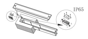
4. PUSH THE FIXTURE INTO THE RECESSED BOX. Make sure the screws be fixed tightly.
