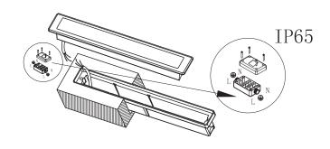
4. PUSH THE FIXTURE INTO THE RECESSED BOX.
