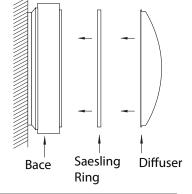
4. Push the Cover Ring into the Bace make sure the screws be fixed tightly..
