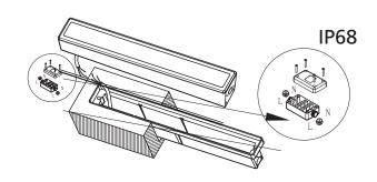
4. Connect the cable connectors of two fixtures in parallel circuit for those wall washers nearby
