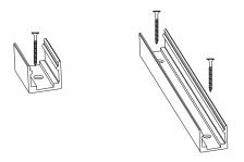
3- Put the parts of the strip light inside the channel / clip and make sure the shiny surface is facing up. using the palm of one hand while using the other hand to gently guide the rest of the strips.
