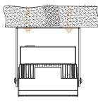
3. After the lamp is installed, the appropriate angle can be adjusted, and the adjustable angle can be adjusted between 0-180°.
