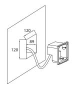
2. Place the Recessed Box and fix it with provided screws
