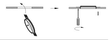
Plaster ceiling surround downlight Buid-in fitting before mounting downlight into housing
