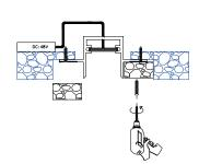
4-(C) Brush the gap between the ceiling on the track and make sure it does not fall into the track. And clean up all the debris in the track.
