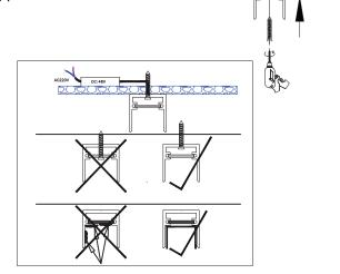
3. by pushing the lamp it will be fixed to the track by magnets
