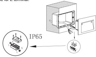
4. PUSH THE FIXTURE INTO THE RECESSED BOX. And fix it with the provided screws
