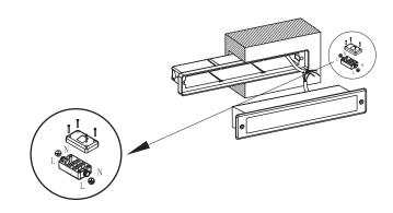
4. PUSH THE FIXTURE INTO THE RECESSED BOX. Make sure the screws be fixed tightly.
