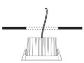
3. PUSH THE FIXTURE into the opening
