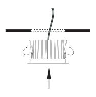
4. CONNECT THE POWER SUPPLY, light up the lamp.
