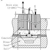
2. FIX THE FLANGE TO THE GROUND. Be sure to fasten the flange tightly.
