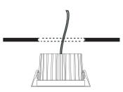
3. PUSH THE FIXTURE into the opening
