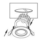
5. PUSH THE FIXTURE into the opening
