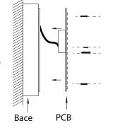
4. Push the Cover Ring into the Bace make sure the screws be fixed tightly..
