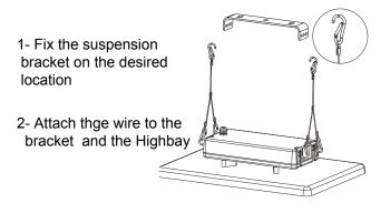
3. Connect the LED Hilux Highbay light into the power outlets and use a waterproof IP65 connector to make sure the fixture is protected.
