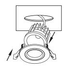
5. PUSH THE FIXTURE into the opening
