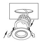
5. PUSH THE FIXTURE into the opening
