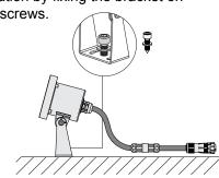
ADJUST THE TILT OF THE LIGHT for a suitable direction for your application.
