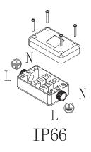
4. Connect the power supply, light up the lamp.
