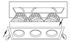
5. PUSH THE FIXTURE into the opening
