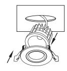
5. PUSH THE FIXTURE into the opening
