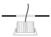
3. PUSH THE FIXTURE into the opening
