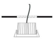
3. PUSH THE FIXTURE into the opening
