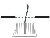
3. PUSH THE FIXTURE into the opening
