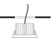
3. PUSH THE FIXTURE into the opening
