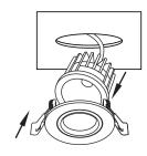
5. PUSH THE FIXTURE into the opening
