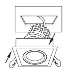
5. PUSH THE FIXTURE into the opening
